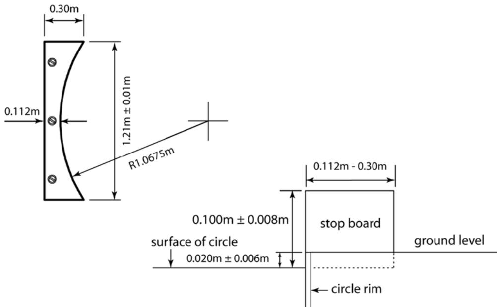
**Figure TR33 (Rule 188) - Shot Put stop board (top and side view)**
