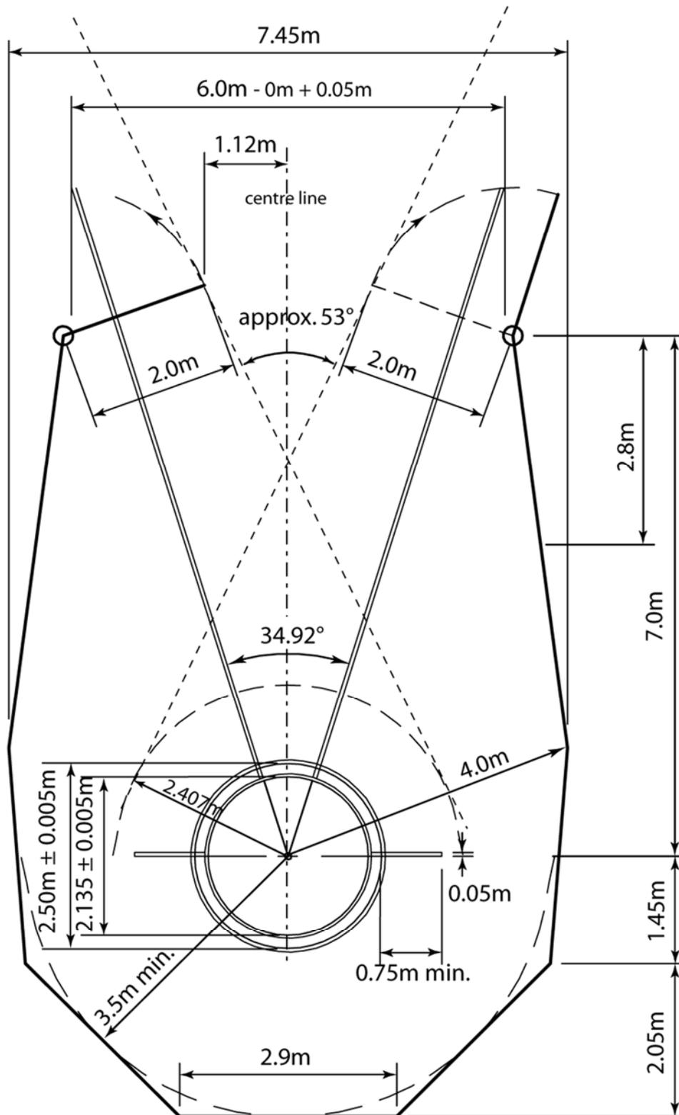
**Figure (a) TR37 (Rule 192) - Cage for Hammer and Discus Throw with concentric circles**
