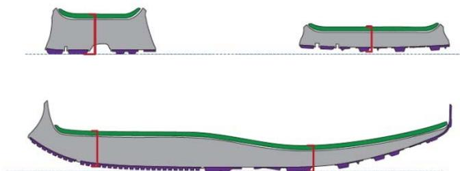
*Note (ii): The centre of the forefoot is the centre point of the shoe at 75% of its internal length. The centre of the heel is the centre point of the shoe at 12% of its internal length. See Figure (b), below. For a standard sample unisex size 42 (EUR), the centre of the forefoot will be the centre point of the shoe approximately 203mm from the inside back of the shoe, and the centre of the heel will be the centre point of the shoe approximately 32mm from the inside back of the shoe.*
